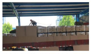
检查时司机没有系安全带,当绳长大于车高时,起不到作用 The driver does not fasten his seat belt during the inspection, When the rope is longer than the height of the car, it does not work
